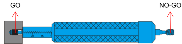
check GO and NO-GO while measuring depth of thread holes
